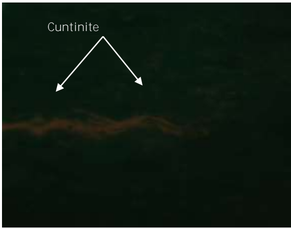
Figure 6. Pyrite and cutinite associated with densinite in coal, reflectant white fluorescence, 500x. Sample 6102/16
