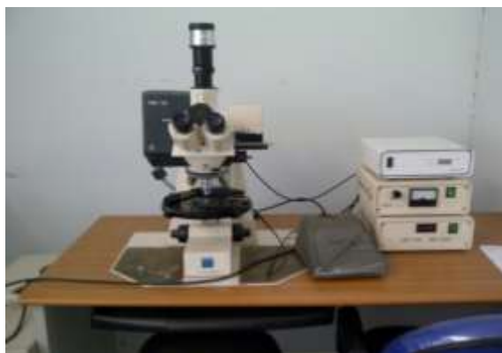
Fig1. Carl Zeiss Microscope and Point Counter Model F with 500 x magnification
