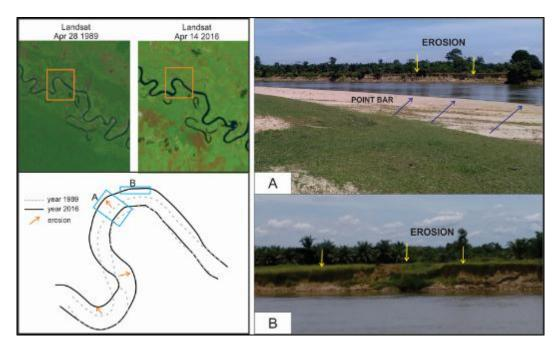
Fig 1. (A) Satellite image that showing geometrical changes the position of the river and image of point bar as result from river migration, and (B). Erosion at the nothern side of the river.
