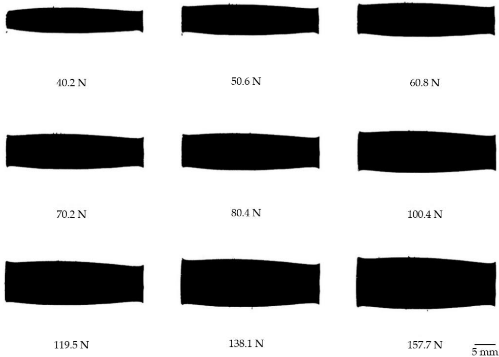
Figure 4. Images of rubber specimen apparent contact area due to applied load (the images belong to trial 2)
